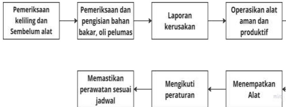
**Gambar 1. Flowchart Alur tugas operator**
