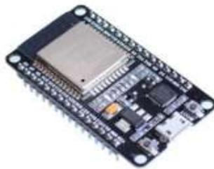
**Figure 1. ESP 32 Microcontroller**
